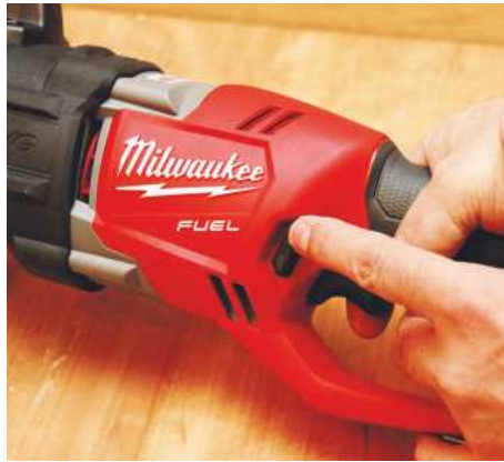
▲ There's an easily operated push-through forward/reverse switch
